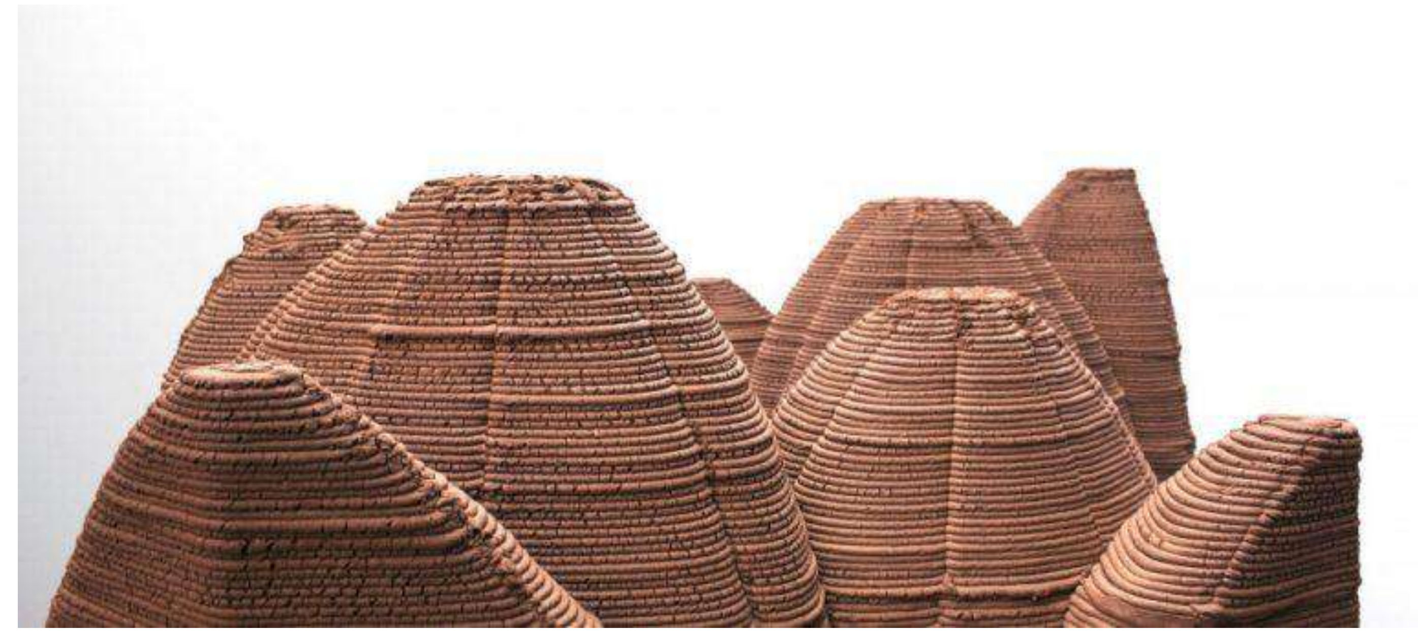
1. 3D printing vaults and domes, by Brenda Freitas and Nitha Shivapuram, 3dPa 2020/21
