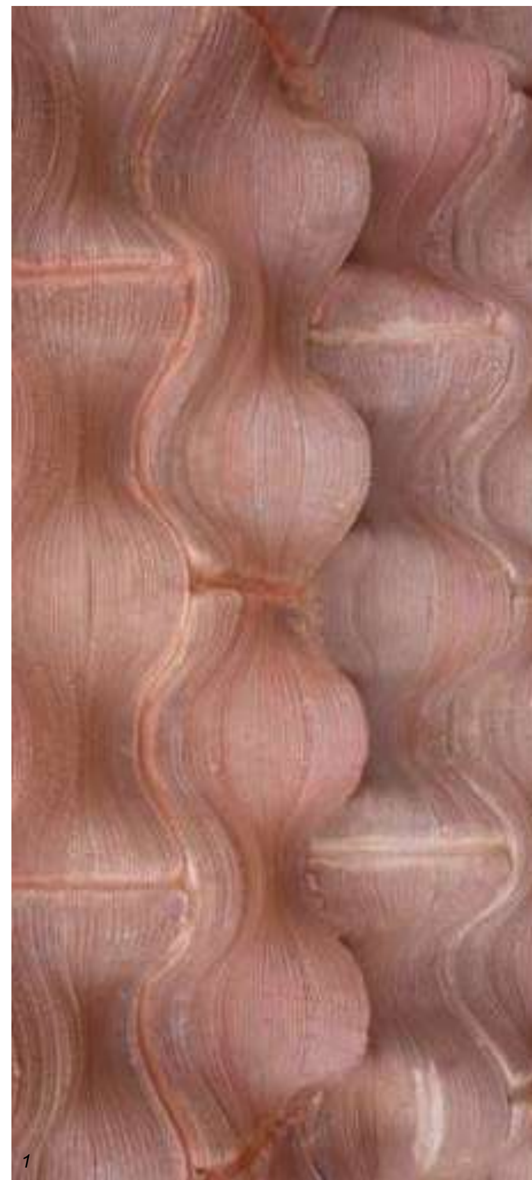
1. Digital Adobe, Cavity network within 3d printed earth wall, collective prototype, 3dPA 2017/18
